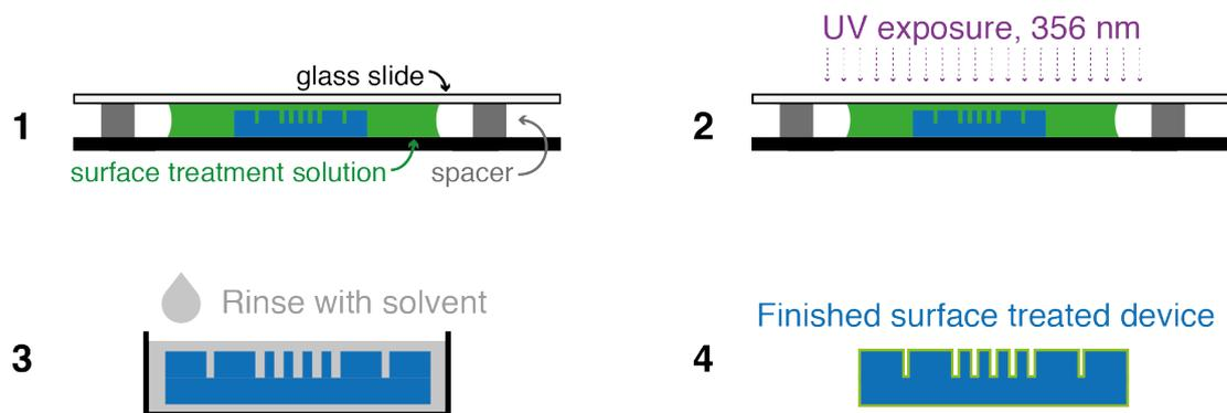
Incubate the device in the surface treatment solution, covering the solution with a glass slide or other transparent layer in order to prevent oxygen inhibition during grafting. Expose to UV, approximately 300s for  $10 \text{ mW/cm}^2$ . Rinse with the same solvent used in the surface treatment solution (normally isopropanol for hydrophilic treatments, and toluene for hydrophobic treatments). Dry in air or by airgun.
