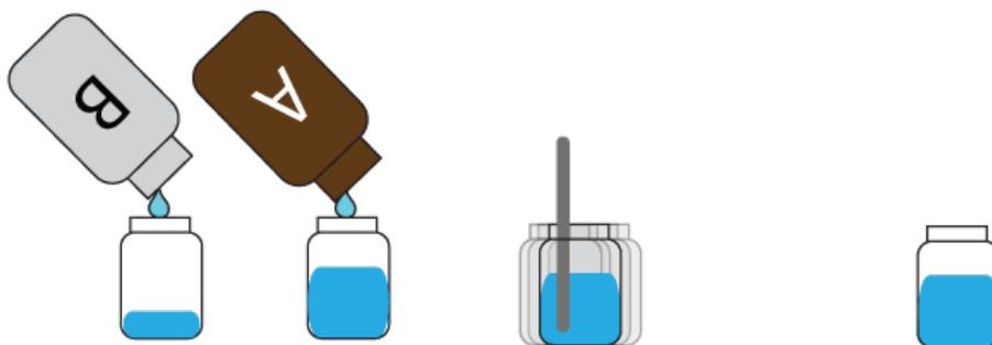
**1** Mix the components      **2** Mix thoroughly      **3** Bubble free in minutes
